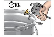
**Turn the Prime Valve knob** forward to the SPRAY position.
