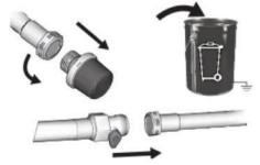
TO SAVE PAINT IN HOSE: Trigger gun into paint pail, turn Prime/Spray Valve forward to SPRAY and turn Power Switch ON. When water comes out of gun, keep gun triggered and aim into waste pail. Continue to flush until water runs clear.
