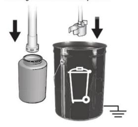
Turn Prime/Spray Valve down to **PRIME**. Turn Power Switch **ON**. Turn Pressure Control Knob to Prime/Clean setting.
