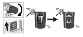
Turn Pressure Control Knob to lowest setting and release trigger. Turn gun trigger lock to locked position. Turn Prime/Spray Valve down to **PRIME**. Turn Power Switch **OFF**.
