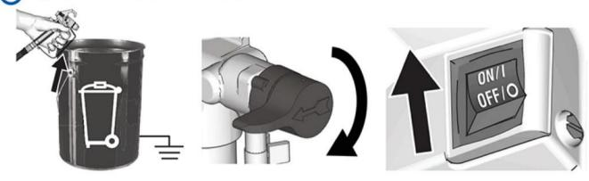
3 When paint comes out of the gun, release trigger. Turn gun trigger lock to locked position. Thread spray tip and quard assembly to gun.
