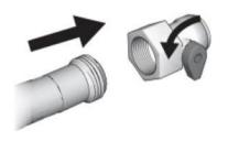
Unscrew inlet strainer from suction tube and place in waste pail for cleaning. Thread Power Flush attachment to suction tube. Turn Power Switch ON and let water run through drain tube for 20 seconds. Turn Power Switch OFF.
